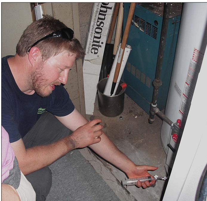
Flint Kinkade of Viridian Energy, a project collaborator, demonstrates vapor sampling technique with a syringe. (Photo courtesy of Jim Rice)
