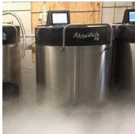
Above F6: The new fancy Abeyance freezers. A lot of vapor was generated during the fill of these 'warm' units.
