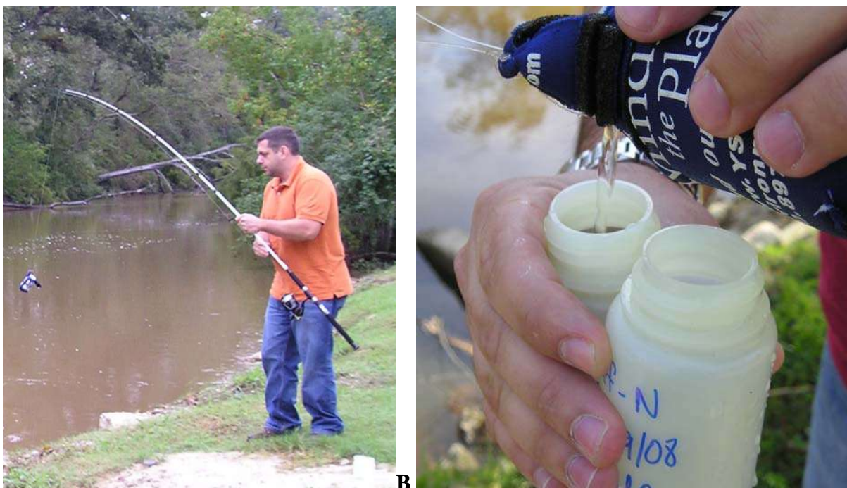
Figure 2: (A) Surface water sampling device and (B) transferring the sample into bottles to take back to the Geochemistry Laboratory at the University of New Orleans.
