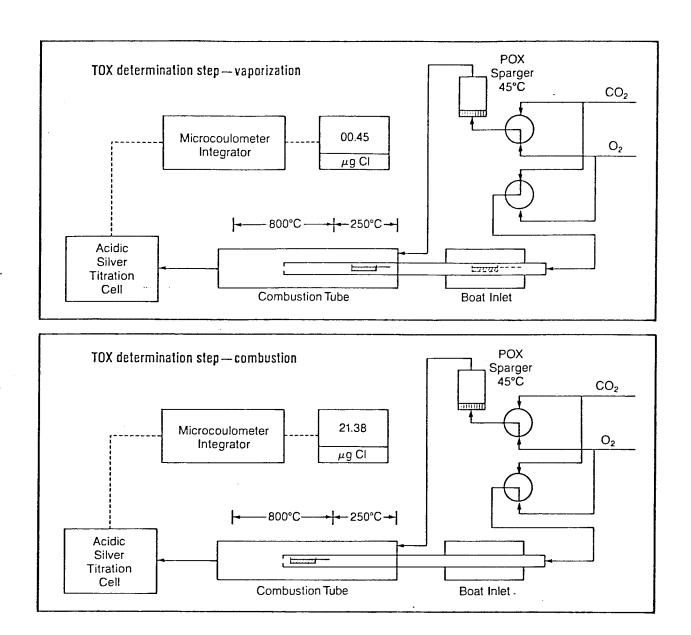
Figure 1. Total organic Halide (TOX) Instrumentation.
