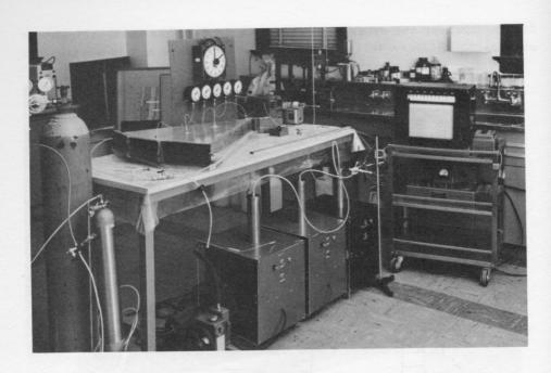
Figure 4.8 GENERAL ARRANGEMENT OF THE RADIAL MINIAQUIFER AND ASSOCIATED EQUIPMENT
