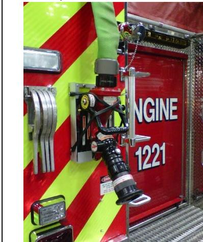
**Figure E:** 500 gpm “fast attack” ground monitor – one intake for 2½” coupled 2½” or 3” hose
