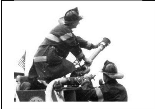
**Figure A - Above:** older style “multiversal appliance” deluge gun supplied by multiple hoselines on top of a pumper
