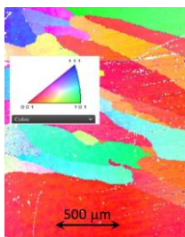
EBSD image showing large grain growth of CrCoFeNi
