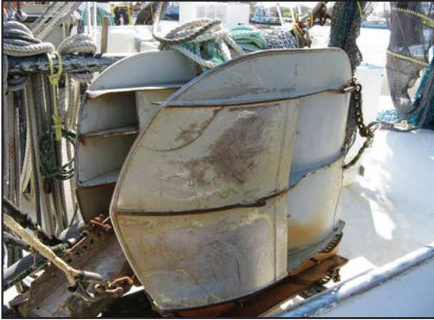
Fuel-saving steel cambered trawl doors
