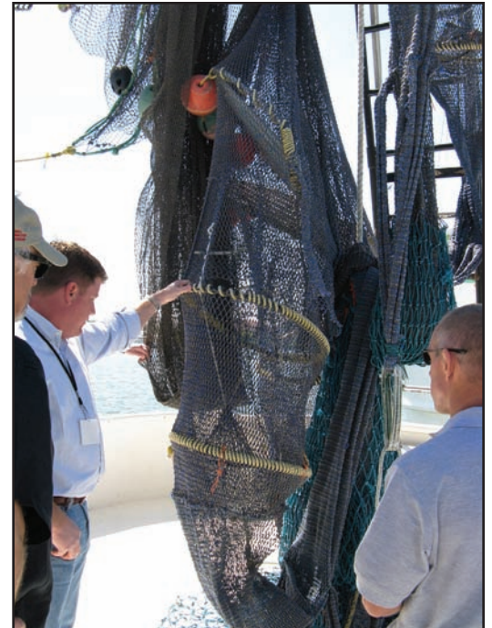
Modified Jones-Davis bycatch reduction device, one of five BRDs approved by NMFS for vessels trawling in federal waters.
