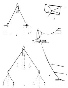
Equipment for directing horizontal shearing: (a) Shearing boats with troll lines for mackerel in the Bay of Kiel, Germany; (b) otterboard for mackerel lines" (c) mackerel fishery with otterboards; (d) Swiss "Seehund" (seal) for troll lines for catching sea-trout
