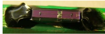
GMR chip with microfluidic structure mounted onto diving board and wire-bond connected. The wires are protected with epoxy glue.
