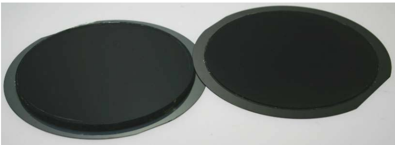
Figs. 4: Silicon wafer with TiOx seed layer and PMMA resist of 650 \mu\text{m} and 1mm, resp., (left); 4" silicon nitride membrane mask with different column designs routinely used for exposures at CAMD and BESSY (1 \mu\text{m} thick membrane with \sim 10 \mu\text{m} thick Au).
