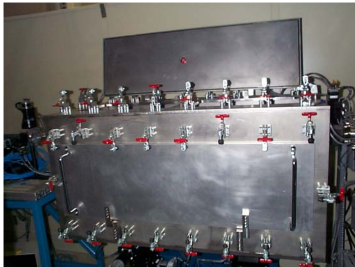
Figure III.B.b.8 GIXAFS vacuum enclosure.
