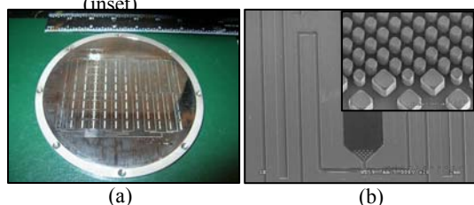
Figure 3: (a) Photomicrograph of the 6-inch LAMI in a stainless steel fixture; and (b) SEM images of hot embossing results: an overall view of a capture bed and a close-up view (inset).
