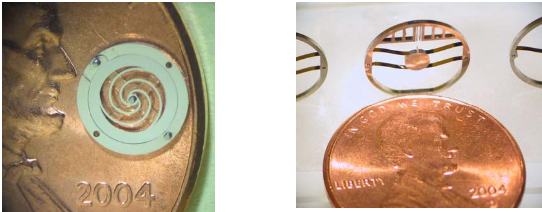
Figs. 2: Precision mechanical switching devices made from NiFe alloy; acceleration switch (left) and acceleration sensitive latching surety components (right).
