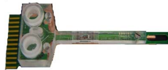
Fluidic cartridge providing an interface between microfluidic channels and macroscopic fluidic connectors.
