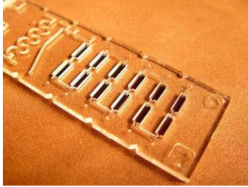
Fluidic test chip with 10 GMR chips prepared with different surface coatings for screening tests.
