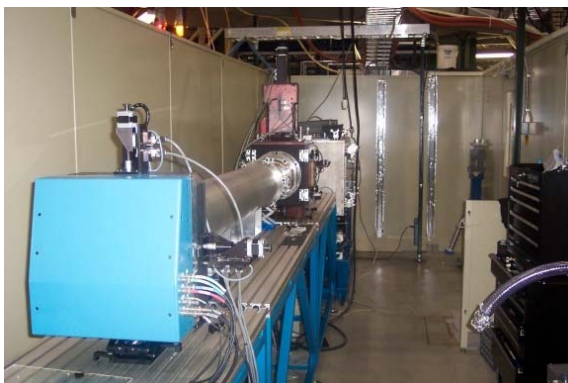
Figure III.B.b.7 SAXS beamline in small angle (left) and wide angle (right) configuration.
