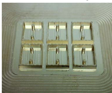
Fig. 4d: Micromachined brass mold.
