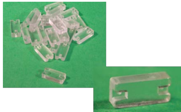
Fig. 5c: Molded fluidic caps (PMMA) with lateral ports to accommodate tubing.
