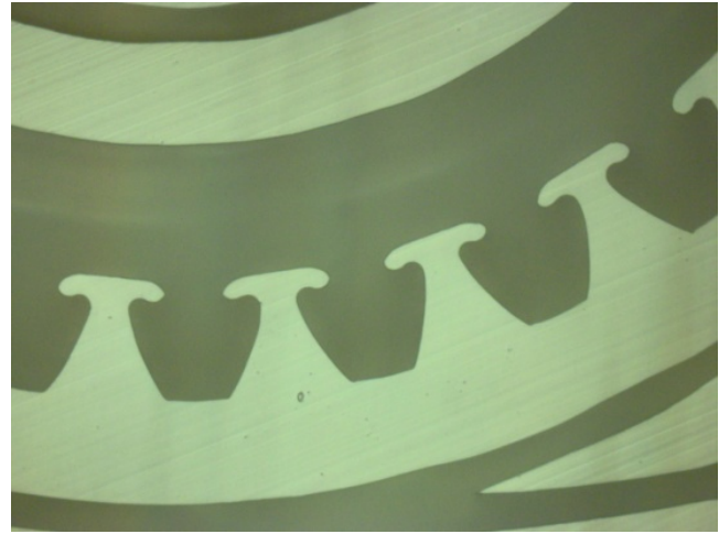
Figure 14b: Optical micrograph of 1mm tall PMMA gear in cell 50 (center of the mask) exposed with 30 \mu m Al filter, no chopper at CLS SyLMAND beamline (test 2).
