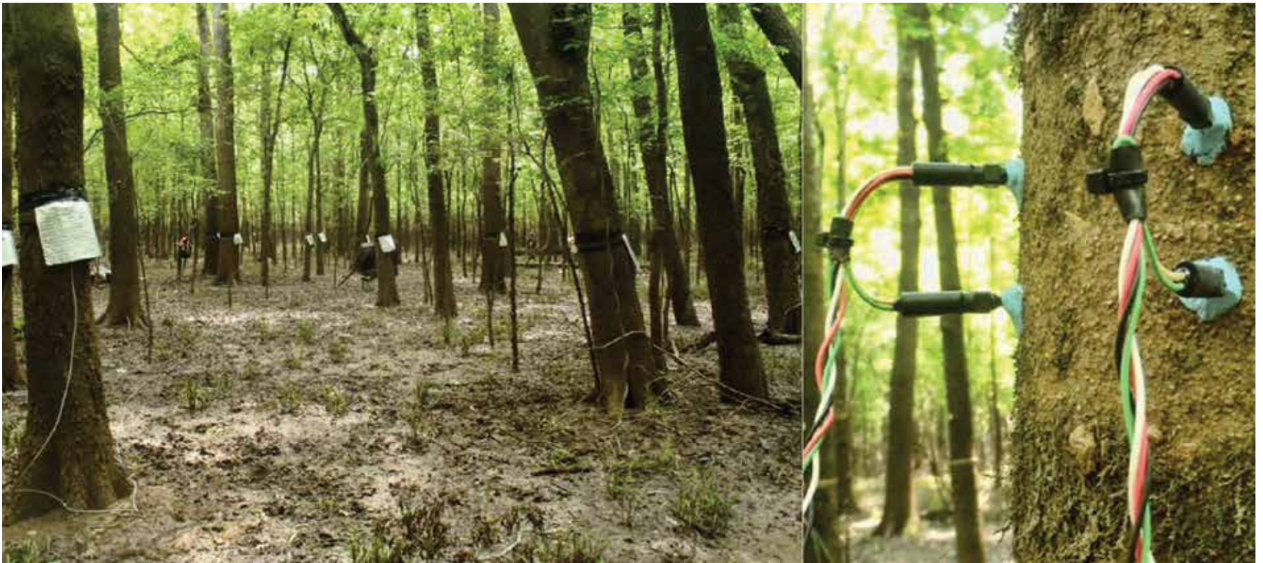
Wired Forest: Thermal Dissipation probes use heat to measure the rate of water flow in trees (White River, Arkansas).
