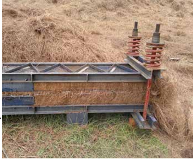
Equipment used to compress pine needles for densification.
