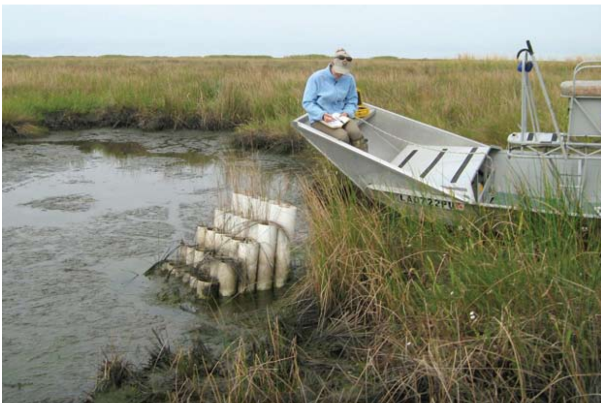
Dr. Vanessa Tobias collects data at Marsh Island Wildlife Refuge. Below her is a "marsh organ," which is used to create a range of flooding conditions for marsh vegetation. The lowest row of plants was continually flooded, while the highest rows seldom flooded.
