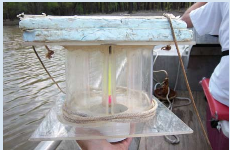
An underwater light trap, used to collect larval fish and invertebrates for the Mollicy Farms project. A light stick in the middle of the trap attracts larval fish and invertebrates during the night. The trap and collected organisms are retrieved the next day.
