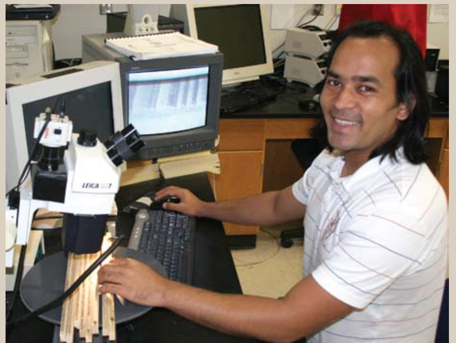
Som Bohora, M.S. student from Nepal, examines baldcypress tree cores for tree-ring measurements on a Velmex measuring stage. Radial growth is assessed in relation to historical changes in climate and hydrology.
