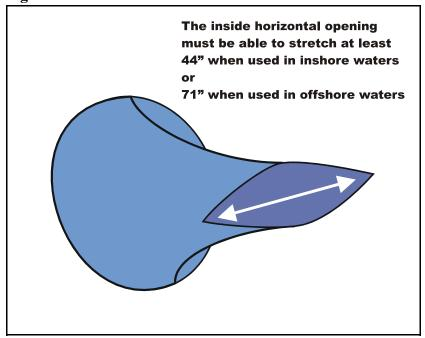
Figure 9 Accelerator funnel attachment
