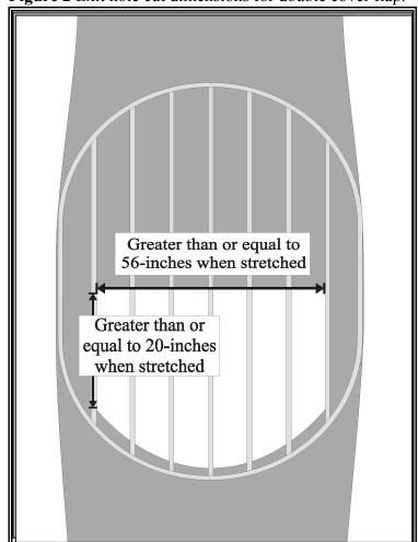
Figure 2 Exit hole cut dimensions for double cover flap.
