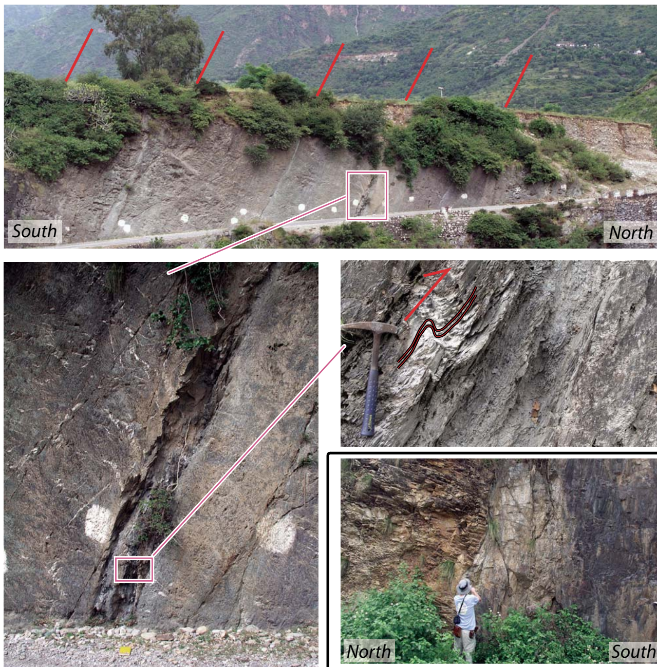
Figure 8. Tons Thrust exposures in the study area. Main frame of photos shows details from an ensemble of brittle faults at the position of Valdiya's (1980) Tons Thrust, along the Bhagirathi River ( 30^{\circ}27'11.4'' , 78^{\circ}25'10.7'' ). Inset photo at bottom right shows the Tons fault juxtaposing slates and quartzites along the Alaknanda River ( 30^{\circ}14'23.1'' , 78^{\circ}49'29.7'' ).
