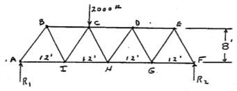
1. Given: The simply supported truss shown is loaded by a 2000# vertical load at point C.
