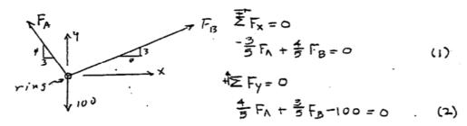
Solve Equas. (1) + (2) simultaneously for FA & FB:
