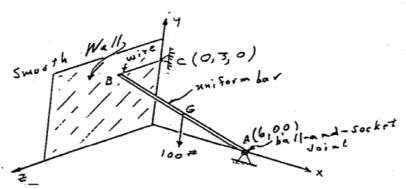
5. Given: A 100# uniform bar AB is supported by a ball-and-socket joint at point A(6,0,0) and by a smooth wall at point B(0,3,2). A wire BC prevents motion.
