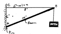
Given: A boom and wire assembly supports a 100 pound weight.
