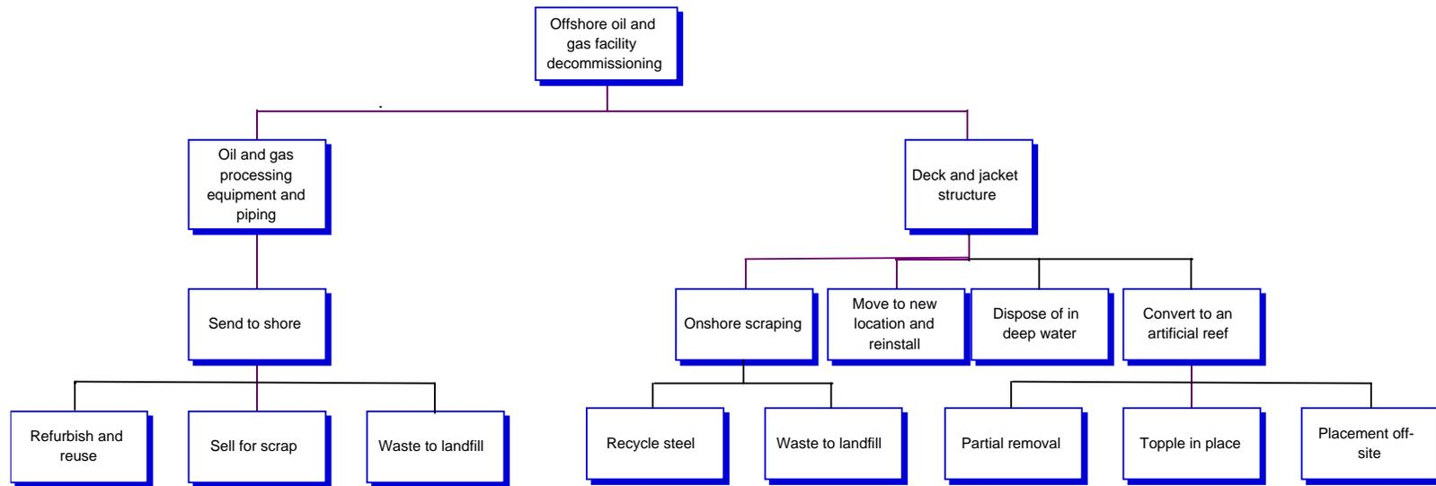
**Figure C.10. Offshore Oil and Gas Facility Decommissioning Tree.**
