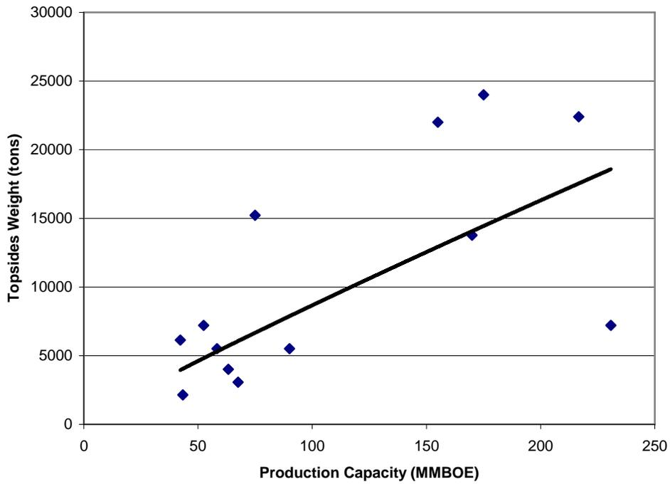
**Figure E.10. TLPs Topsides Weight as a Function of Production Capacity.**
